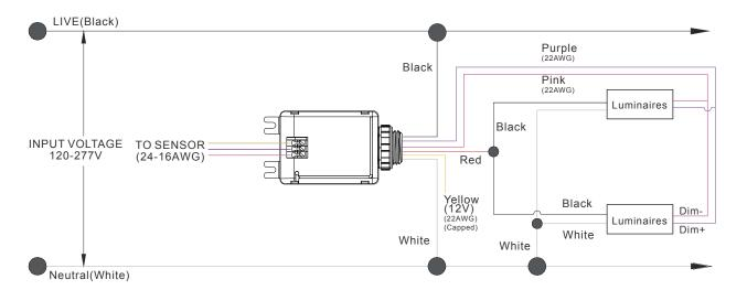
\* Please make sure the 0-10V dimming current not exceeding the Max. sinking current of the sensor when multiple fixtures connecting to the sensor that power by BMWC-L103S.
